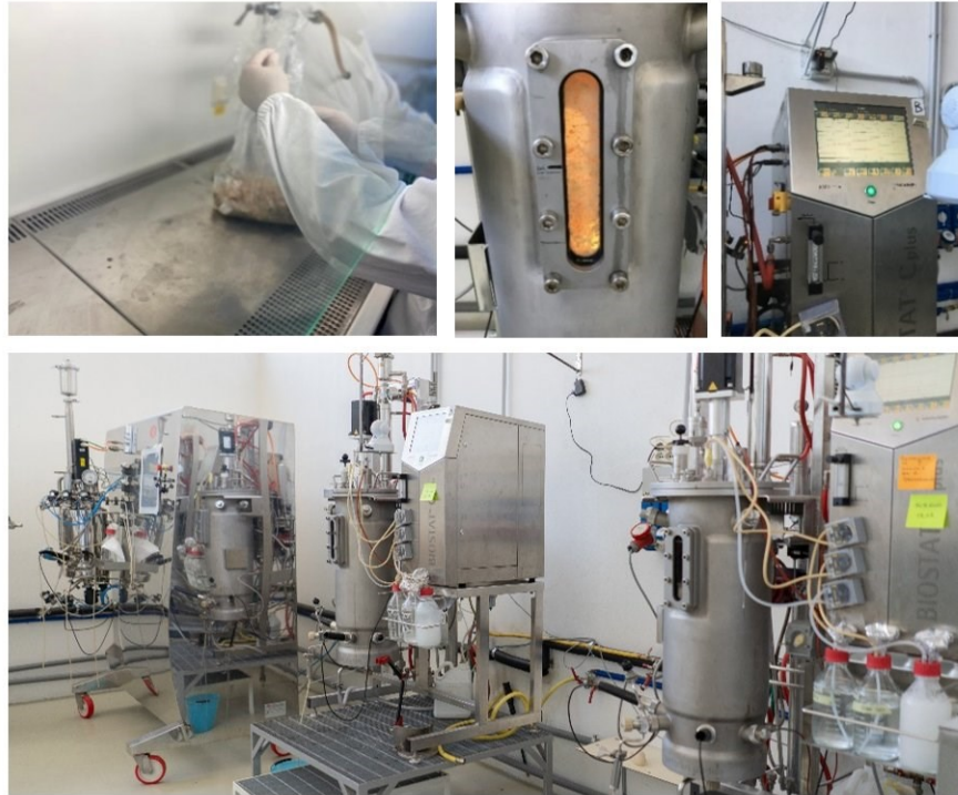
Figure 32. Production of P. chlamydosporia on static bioreactors with intermittent air flow.
