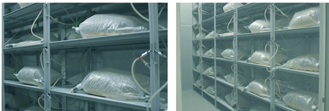
Figure 2. Downstream mass production of P. chlamydosporia on solid medium.
