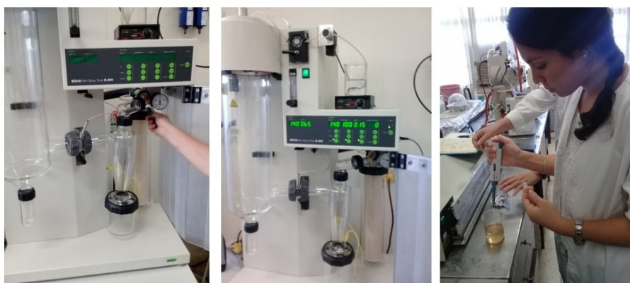
Figure 31. Spray drier equipment available at CENSA and used for a preliminary study on IJ formulation.
