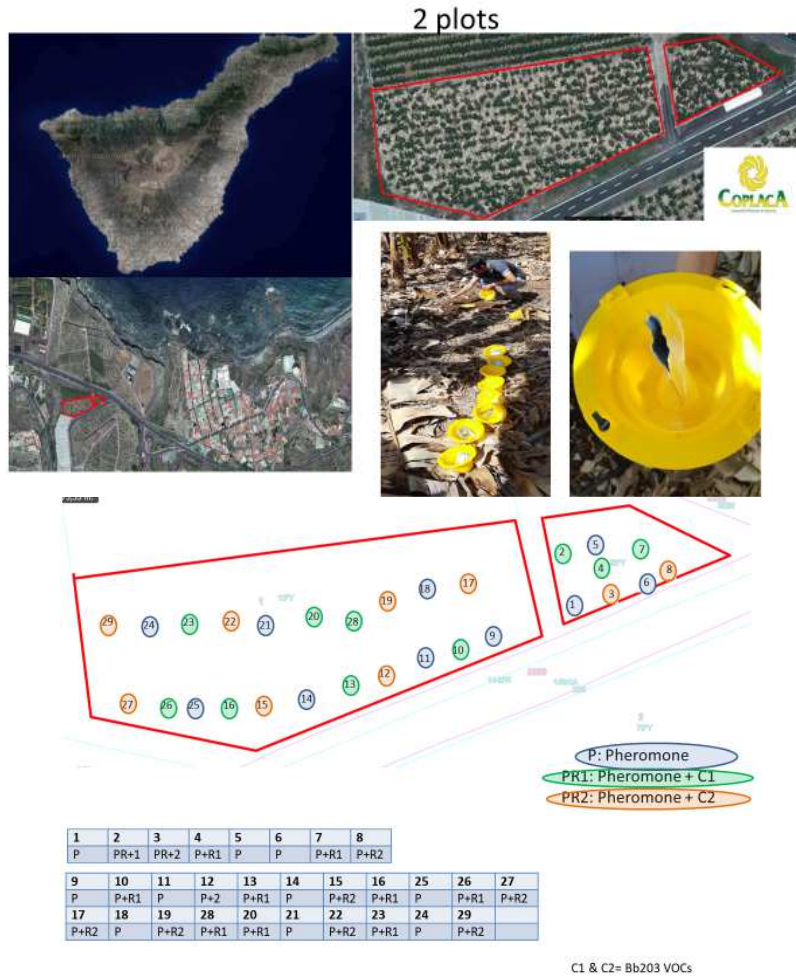
Figure 34. Field testing of VOCs on BW.
